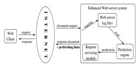
Figure 1: Proposed architecture of a predictionenabled Web server.
