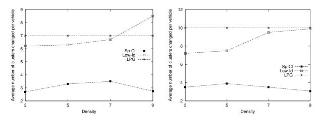
Fig. 10. Average cluster change per vehicle for Sp-Cl, LPG and Low-Id methods for different transmission ranges (125m, 80m).
