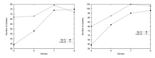
Fig. 11. The average total number of formed clusters for Sp-Cl and Low-Id methods for different transmission ranges (125m, 80m).
