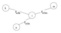
Fig. 2. Relative forces applied to vehicle *i*.
