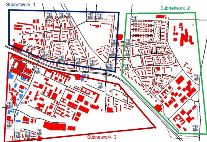
Figure 4.1: City is divided in subnetworks. RSUs are located in entries/exits of each subnetwork.
