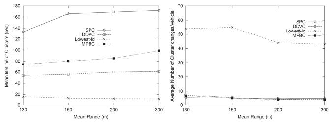
Fig. 11. Lifetime and mean cluster changes versus range.
