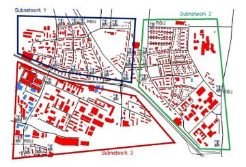
Fig. 1. City is divided in subnetworks. RSUs are located at the entrances/exits of each subnetwork.
