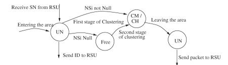
Fig. 7. States of a vehicle.
