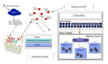
Fig. 4: NITOS testbed: a cloud based, service oriented wirelss testbed facility
