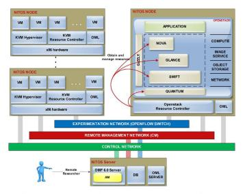
Fig. 2: NITOS testbed: Cloud Management Architecture
