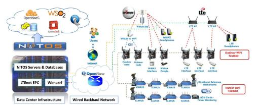
Fig. 1: NITOS testbed: a cloud based, service oriented wirelss testbed facility
